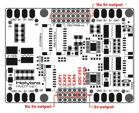
\* Note: In order to power servos, the 8-pins power (+) rail of **FMU PWM-OUT** needs to be connected to a BEC equipped ESC or a standalone 5V BEC or a 2S LiPo battery. Be careful with the voltage of servos you are going to supply here.
