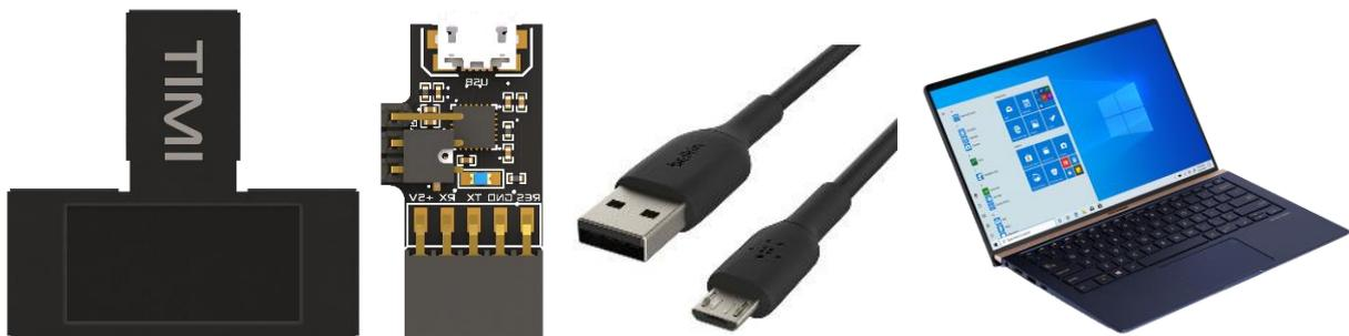
The BBM-Programmer does not come with the microUSB cable, this can be purchased from virtually any hardware/computer store.
