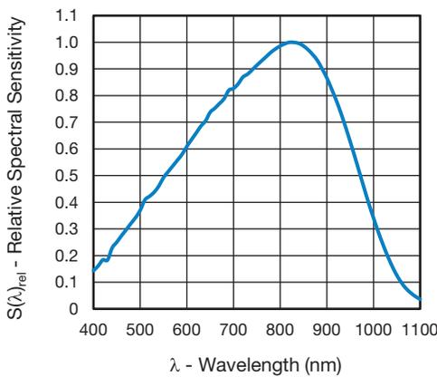
Fig. 7 - Relative Spectral Sensitivity vs. Wavelength (Biosensor)
