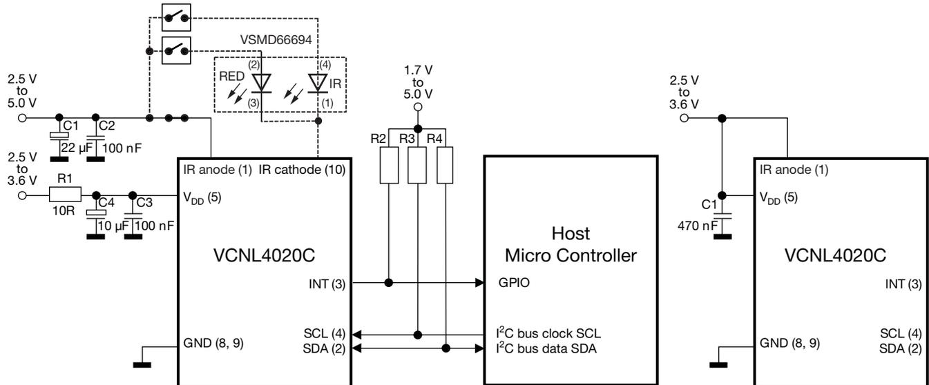
Fig. 12 - Application Circuit (x) = Pin Number
