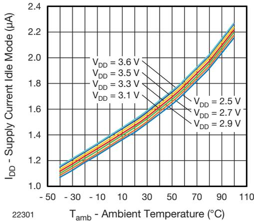
Fig. 1 - Idle Current vs. Ambient Temperature
