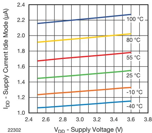
Fig. 2 - Idle Current vs. V<sub>DD</sub>
