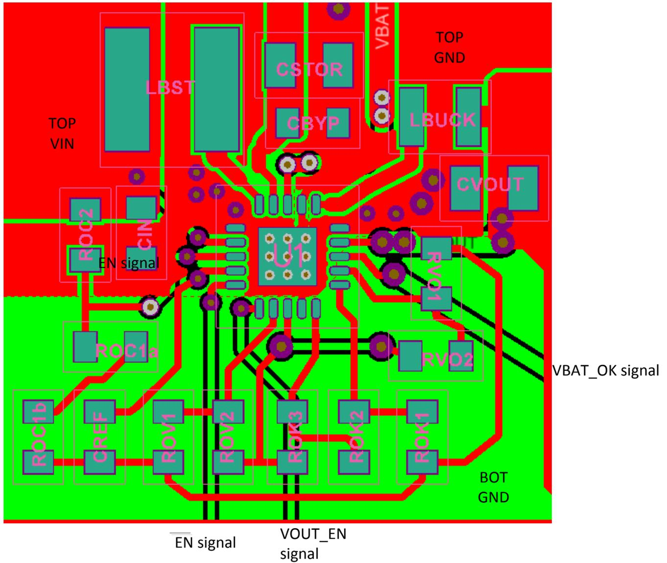
Figure 48. Layout Schematic
