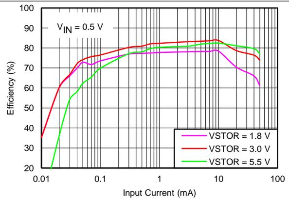
$V_{IN\_DC}$  = sourcemeter configured with voltage source = 0.5 V and  $I_{COMP}$  varied from 0.01 mA to 100 mA
