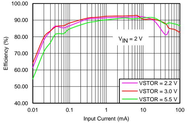
$V_{IN\_DC}$  = sourcemeter configured with voltage source = 2.0 V and  $I_{COMP}$  varied from 0.01 mA to 100 mA
