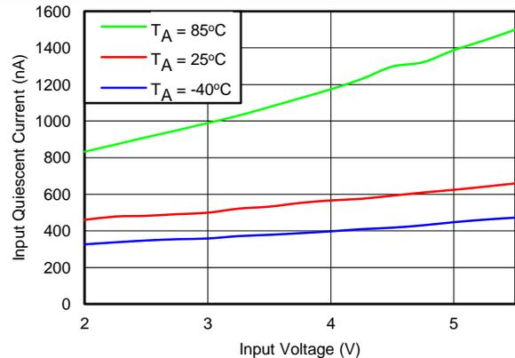
$V_{IN\_DC}$  = floating and  $\overline{EN} = V_{OUT\_EN} = GND$
