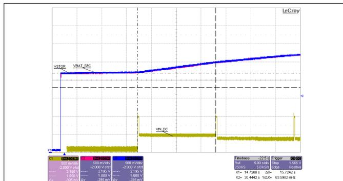
Sourcemeter with  $V_{SOURCE} = 1.0 \text{ V}$  and compliance of  $8.5 \text{ mA}$  subsequently applied to  $V_{IN\_DC}$
