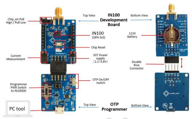
Figure 49 Programming with NanoBeacon<sup>™</sup> config tool
