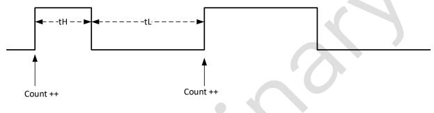
Figure 37 GPIO edge counting
