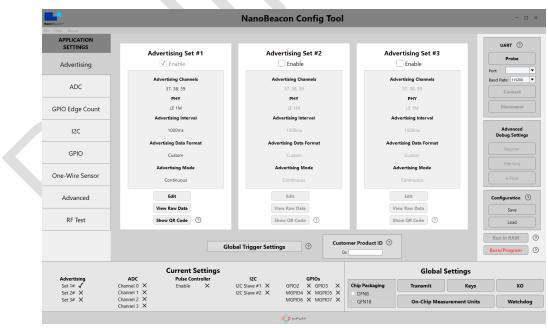
Figure 2 NanoBeacon config PC GUI tool
