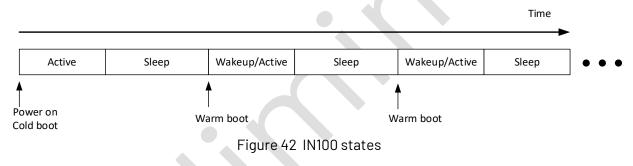
Execute I2C command when cold boot: Execute I2C read/write command when cold boot. If only this execution condition is checked, then the corresponding I2C command will be executed only once when the chip is cold booted, which is often used for the initial configuration of the I2C device.
