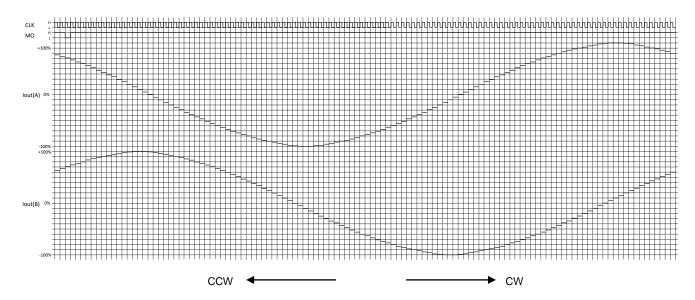
Waveform of MO output: State of pull-up.
