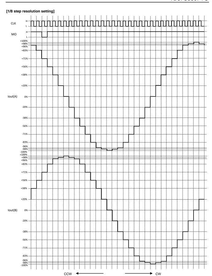
Waveform of MO output: State of pull-up.
