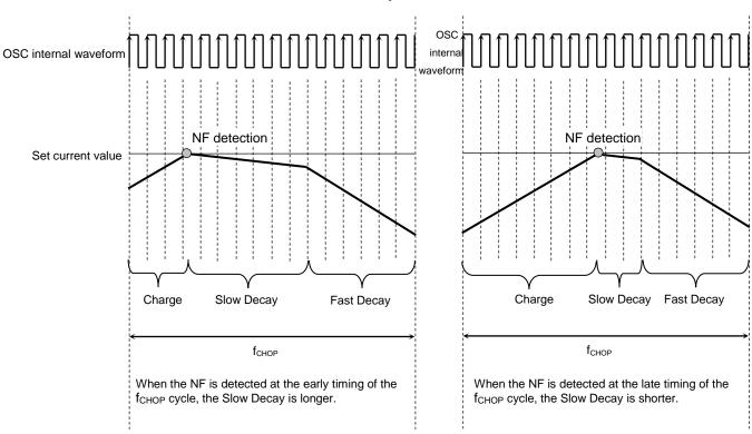
The Charge period (the time until the motor current reaches the set current value) is determined by the operating status. Therefore, the NF detection (the motor current reaches the set current value) timing with in the chopping cycle will change. When the NF is detected at the early timing of the f<sub>CHOP</sub> cycle, the Slow Decay is longer. When the NF is detected at the late timing of the f<sub>CHOP</sub> cycle, the Slow Decay is shorter, as shown above.
