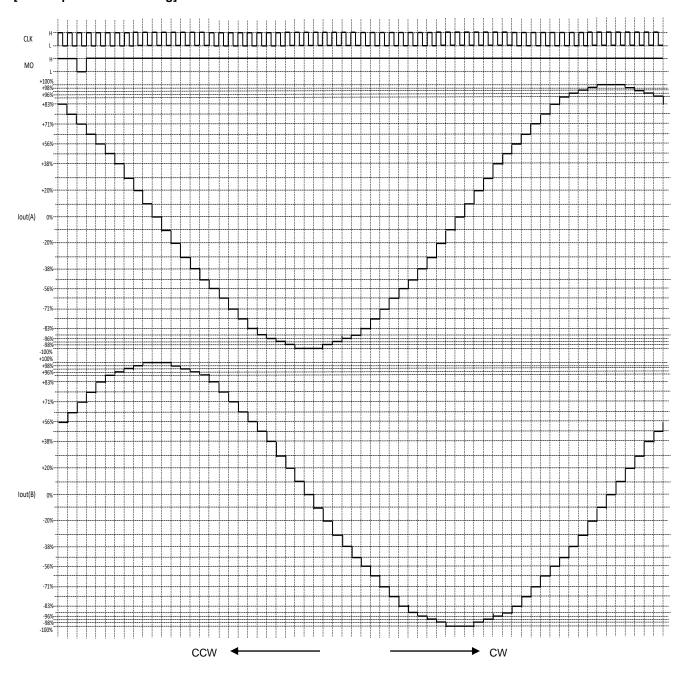
Waveform of MO output: State of pull-up.
