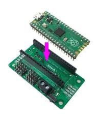
Power is provided via a terminal block connector, the supply is then controlled by an on/off power switch to the board. There is a green power LED to indicate when the board is turned on. The power connections are reverse polarity protected.
