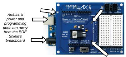
Make sure the BOE Shield mounting holes align with the Arduino module's.
