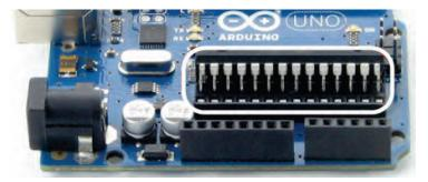
A sketch can make the digital pins send high (5 V) or low (0 V) signals *to* circuits. In this chapter, we'll do that to turn lights on and off. A sketch can also make a digital pin monitor high or low signals coming *from* a circuit; we'll do that in another chapter to detect whether a contact switch has been pressed or released.
