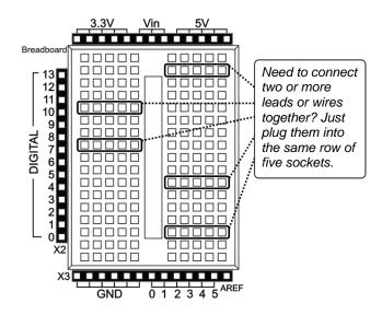
The prototyping area also has black sockets along the top, bottom, and left.
