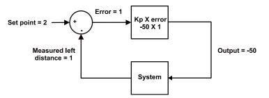
The next time through the loop, the measured distance might change, but that's okay. Regardless of the measured distance, this control loop will calculate a value that will cause the servo to move to correct any error. The correction is always *proportional* to the error. The two calculations involved:
