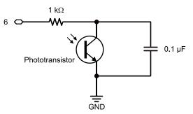
**QT Circuit:** A common abbreviation for charge transfer is QT. The letter Q refers to electrical charge (an accumulation of electrons), and T is for transfer.
