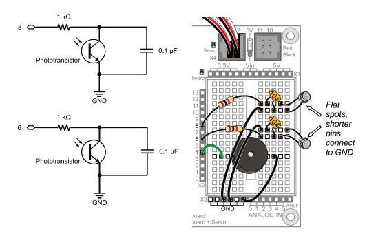
The roaming examples in this chapter will depend on the phototransistors being pointed upward and outward to detect differences in light levels from different directions.
