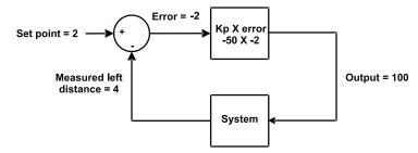
This block diagram could apply to either the left IR distance sensor and servo output or the right. In fact, your code will maintain two identical control loops, one for each side of the BOE Shield-Bot. Let's walk through this example.
