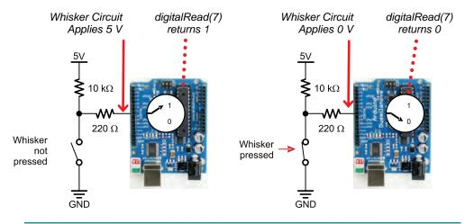
**Switch Lingo:** Each whisker is both the mechanical extension and the ground electrical connection of a normally open (off until pressed) momentary (on only while pressed) single-pole (one set of electrical contact points), single-throw (only one position conducts) switch.
