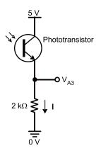
If you replace the 2 k $\Omega$  resistor with a 1 k $\Omega$  resistor, V<sub>A3</sub> will see smaller values for the same currents. In fact, it will take twice as much current to get V<sub>A3</sub> to the same voltage level, which means the light will have to be twice as bright to reach the 3.5 V level, the default voltage in HaltUnderBrightLight to make the BOE Shield-Bot stop.
