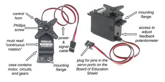
In this activity, you will connect your servos to the Board of Education Shield's servo ports, which will connect them to supply voltage, ground, and a signal pin. You will also connect a battery supply to your Arduino because, under certain conditions, servos can end up demanding more current than a USB supply is designed to deliver.
