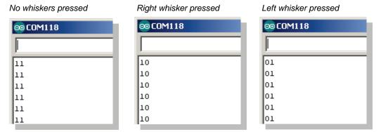
Active-low Output : The whisker circuits are wired for active-low output, which means that they each send a low signal when they are pressed (active) and a high signal when they are not pressed. Since digitalRead returns 0 for a low signal and 1 for a high signal, 0 is what tells your sketch that a whisker is pressed, and 1 tells it that a whisker is not pressed.
