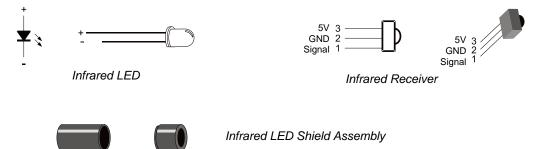
✓ Check the figure below to make sure you have selected infrared LEDs and not phototransistors. The infrared LED has a taller and more rounded plastic dome, and is shown on the right side of this drawing.
