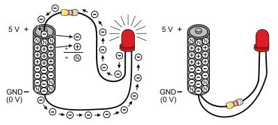
On the left side of the picture, one LED lead is connected to 5 V and the other to GND. So, 5 V of electrical pressure causes electrons to flow through the circuit (electric current), and that current causes the LED to emit light. The circuit on the right side has both ends of the LED circuit connected to GND. This makes the voltage the same (0 V) at both ends of the circuit. No electrical pressure = no current = no light.
