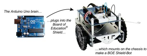
The activities in this tutorial will guide you through building the mechanical parts and circuits that make the BOE Shield-Bot work. Then, you'll write simple programs that make the Arduino and your robot do four essential robotic tasks:
