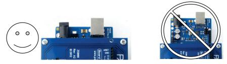
Component placement varies a little bit for the different Arduino models; some can only fit one or two Nylon standoffs for holding the boards together. This is okay, but you need to find out which holes you can use before socketing the Board of Education Shield.
