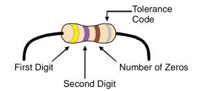
Here's how to find the resistor's value, in this case proving that yellow-violet-brown is really 470  $\Omega$ :
