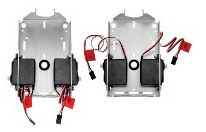
**Outside-forward (left)** — the servos' mounting tabs seat outside the chassis, with their potentiometer access ports facing toward the front of the chassis. This allows easy access to adjust the potentiometers on an assembled robot, and also makes servo replacement quick. However, this gives the BOE Shield-Bot a longer, wider wheel base, so it will be a little less nimble on maneuvers and may need more pulses to make turns.
