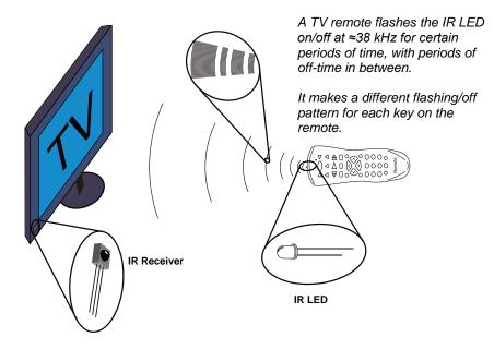
The TV remote sends messages by flashing the IR LED very fast, at a rate of about 38 kHz (about 38,000 times per second). The IR receiver only responds to infrared if it's flashing at this rate. This prevents infrared from sources like the sun and incandescent lights from being misinterpreted as messages from the remote. So, to send signals that the IR receiver can detect, your Arduino will have to flash the IR LED on/off at 38 kHz.
