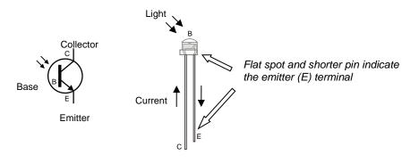
The phototransistor looks a little bit like an LED. The two devices do have two similarities. First, if you connect the phototransistor in the circuit backwards, it won't work right. Second, it also has two different length pins and a flat spot on its plastic case for identifying its terminals. The longer of the two pins indicates the phototransistor's collector terminal. The shorter pin indicates the emitter, and it connects closer to a flat spot on the phototransistor's clear plastic case.
