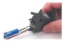
Insert tip of screwdriver into potentiometer access hole,
