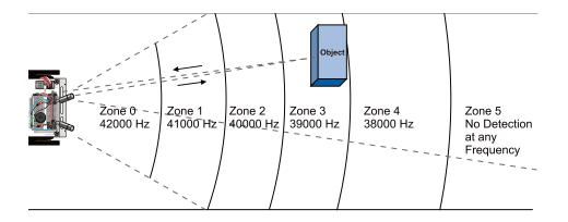
The **irDistance** function from the next sketch performs distance measurement using the technique shown above. Code in the main loop calls **irDistance** and passes it values for a pair of IR LED and receiver pins. For example, the **loop** function uses **int irLeft** = **irDistance(9, 10)** to check distance to an object in the left side of the BOE Shield-Bot's detection zone "field of vision."
