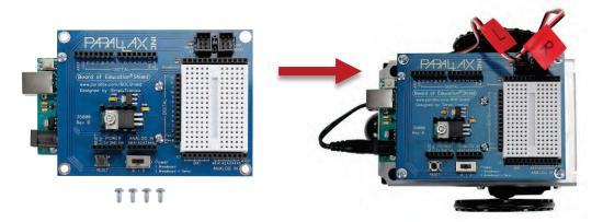
From the underside of the chassis, pull any excess servo and battery cable through the rubber grommet hole, and tuck the excess cable lengths between the servos and the chassis.
