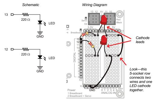
The next picture will give you an idea of what is going on when you program the Arduino to control the LED circuit. Imagine that you have a 5 volt (5 V) battery. The Board of Education Shield has a device called a *voltage regulator* that supplies 5 volts to the sockets labeled 5V. When you connect the anode end of the LED circuit to 5 V, it's like connecting it to the
