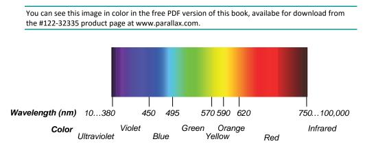
The phototransistor in the Robotics Shield Kit is most sensitive to 850 nm wavelengths, which is in the infrared range. Infrared light is not visible to the human eye, but many different light sources emit considerable amounts of it, including halogen and incandescent lamps, and especially the sun. This phototransistor also responds to visible light, though it's less sensitive, especially to wavelengths below 450 nm.
