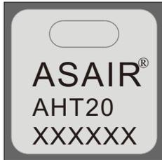
Figure 16: Sensor laser label
