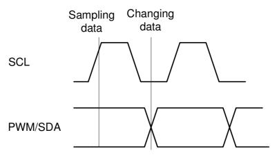
Figure 9: Bit transfer on SMBus
