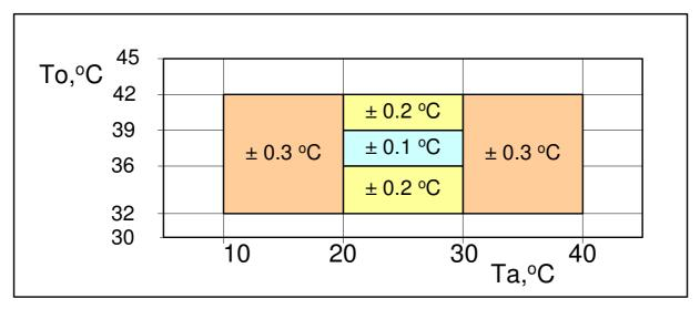
Figure 22: Accuracy of MLX90614DAA (Ta,To) for medical applications. Accuracy of the MLX90614DCH and DCI for VDD = 3V (see paragraph 10.1.3)
