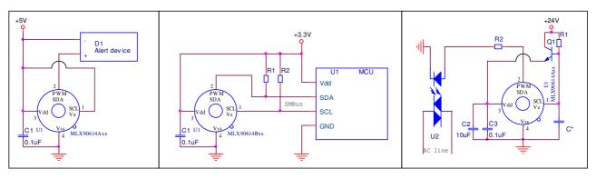
Figure 38: Thermal alert/thermostat applications of MLX90614
