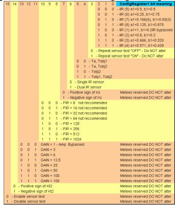
Note: The following bits/registers should not be altered (except with special tools – contact Melexis for such tools availability) in order to keep the factory calibration relevant:
