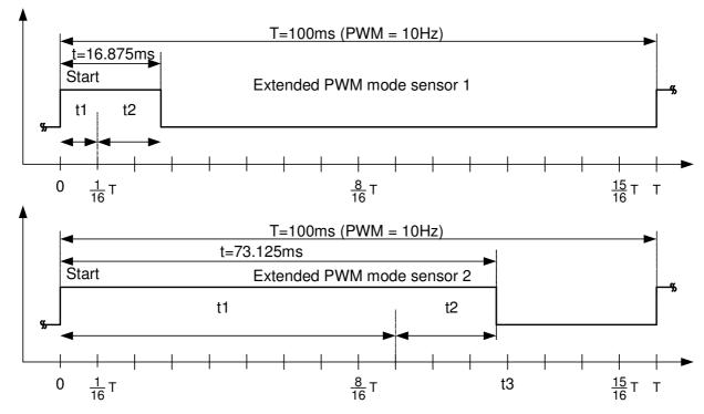
Figure 16: Example: Extended PWM mode readings – sensor 1 above and sensor 2 bellow
