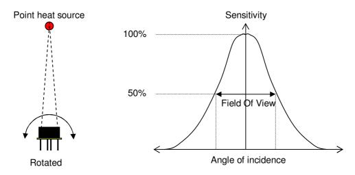
Figure 26: Field Of View measurement
