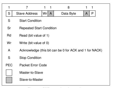
Figure 4: SMBus packet element key
