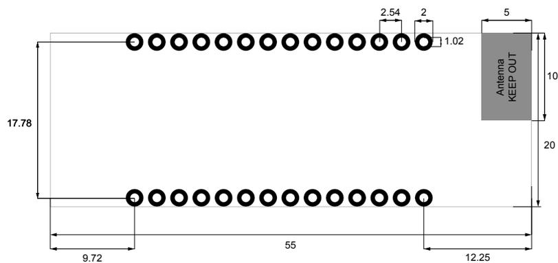
Figure 7 – Recommended land pattern (through hole) – Units: mm
