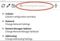
3. Click in the **AT command to search...** field at the top and type **AN** to highlight the Access Point Name (AN) setting. By default there is just a hyphen shown here.
