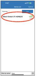
3. You should see your device listed. If the signal is very weak, confirm that the BLE antenna is properly connected. (*The first time you open the app on a phone and scan for devices, the device list contains only the name of the device and the BLE signal strength. After you have authenticated, the IMEI for the device will also appear in the device list.*)
