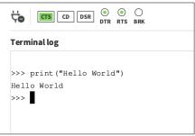
3. Any line of MicroPython code will work, and variables will be stored between commands. Try typing **x** = **2** + **2** then pressing Enter. Finally, type **print(x)** to see the answer.
