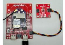
2. Confirm that the switch on the lower left side of the Development Board is in the down position for I2C. If this switch is set incorrectly the sensor will not be able to communicate, so it's very important!
