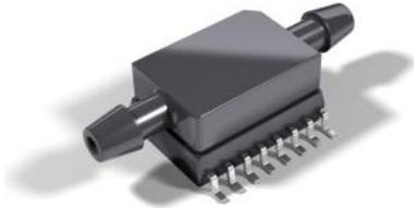
The SM8436 series are digital, ultra-low pressure sensors offering state-of-the-art MEMS pressure transducer technology and CMOS mixed signal processing technology to produce a digital, fully conditioned, multi-order pressure and temperature compensated sensor in JEDEC standard SOIC-16 package with a dual vertical porting option (dual horizontal porting available for selected configurations). It is available in a gage and a differential pressure configuration.
