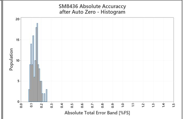
Accuracy at -20Pa to 20Pa tested at 30°C and 5.0V
