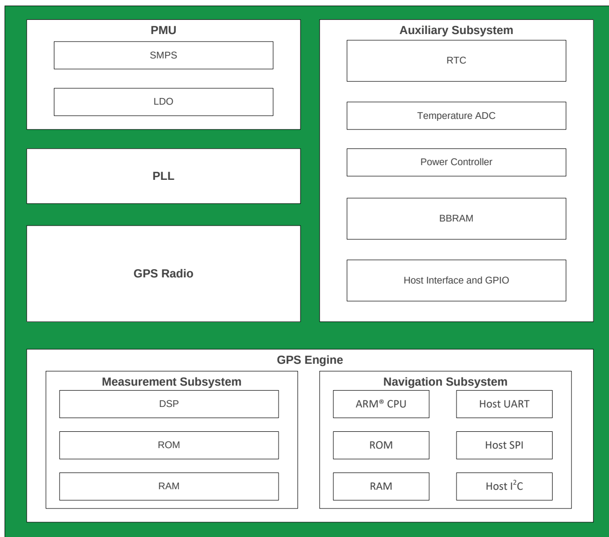
FIGURE 2 – SiRFstarIV™ GSD4e GPS SoC BLOCK DIAGRAM
