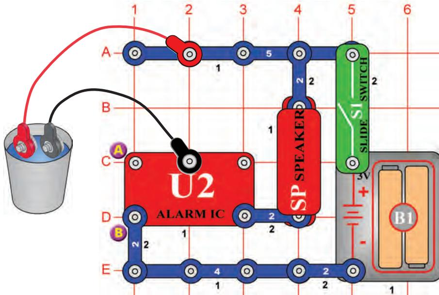
Build the circuit shown but initially leave the jumper wires outside the cup. Turn on the slide switch (S1); nothing happens. Place the jumper wires into a cup of water and an alarm sounds!
