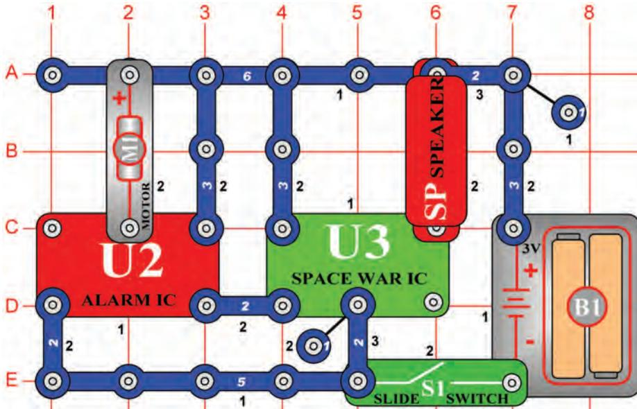
Build the circuit shown on the left, which is based on the circuit in the Space War Project #19. Turn on the switch and you will hear exciting sounds, as if a space battle is raging!
