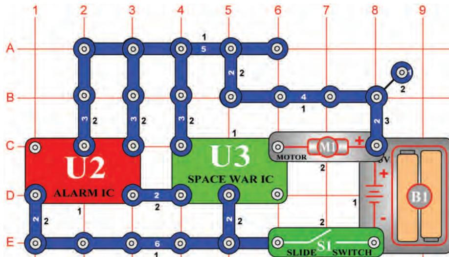
Turn on the slide switch (S1) and the motor (M1) spins (you may need to give it a push with your finger to get it started). The sounds from the space war IC (U3) are used to drive the motor. Because the motor uses magnets and a coil of wire similar to a speaker, you may even hear the space war sounds coming faintly from the motor.
