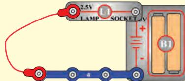
4. **Slide switch (S1) and Press switch (S2):** Build project #1, if the lamp (L1) doesn't light then the slide switch is bad. Replace the slide switch with the press switch to test it.
