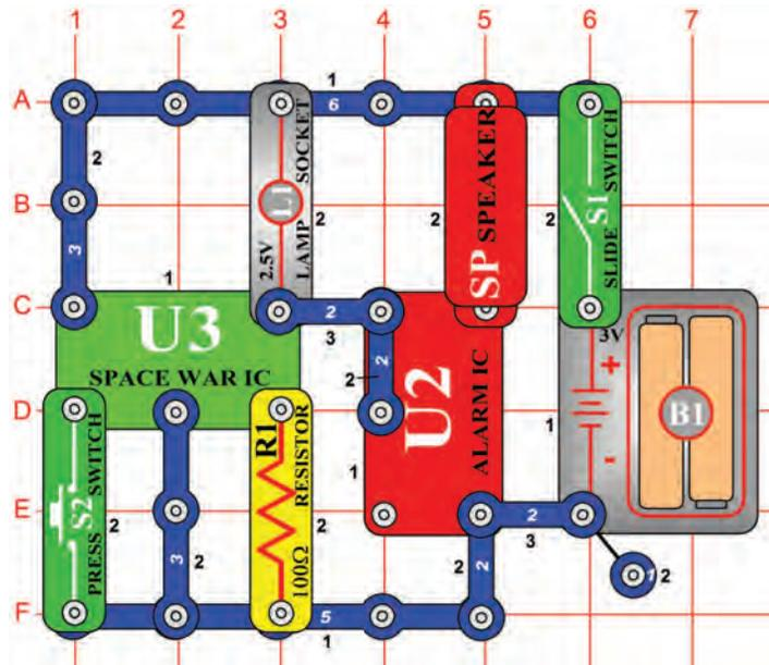
Build the circuit shown on the left and turn on the slide switch (S1). Press and hold the press switch (S2) to make the lamp (L1) brighter.
