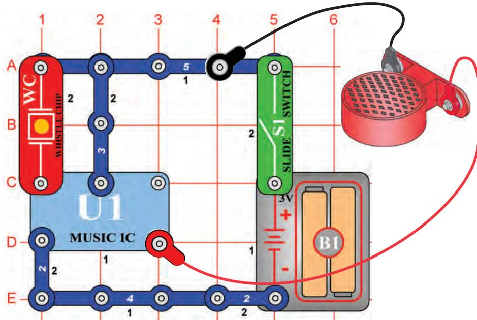
Build the circuit shown on the left by placing all the parts with a black 1 next to them on the base grid first. Then, assemble parts marked with a 2. Finally, lay the speaker (SP) on the table and connect it to the circuit using the jumper wires as shown.
