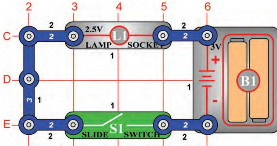
Build the circuit shown on the left by placing all the parts with a black 1 next to them on the base grid first. Then, assemble parts marked with a 2. Install two (2) “AA” batteries (not included) into the battery holder (B1).
