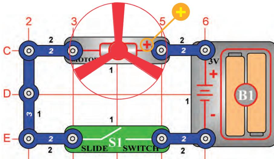
Build the circuit shown on the left by placing all the parts with a black 1 next to them on the base grid first. Then, assemble parts marked with a 2.
