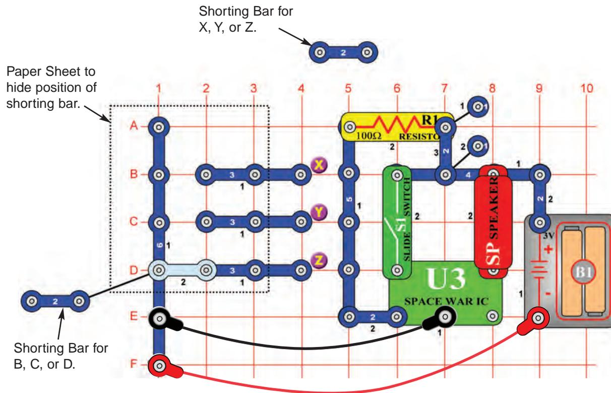
Build the circuit at left. It uses both jumper wires as permanent connections. It also uses two 2-snap wires as “shunting bars”.
