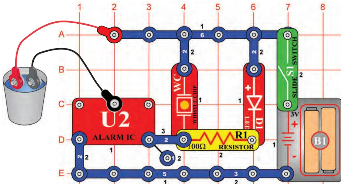
Sometimes you want a water alarm that can be heard but is not loud enough to be annoying or distracting, so let's make one. We'll also put a light on it that could be seen in a noisy room, in a real application you could use a powerful light that would be easily seen. Build the circuit shown but initially leave the jumper wires outside the cup. Turn on the slide switch (S1); nothing happens. Place the jumper wires into a cup of water and an alarm sounds and the light comes on.
