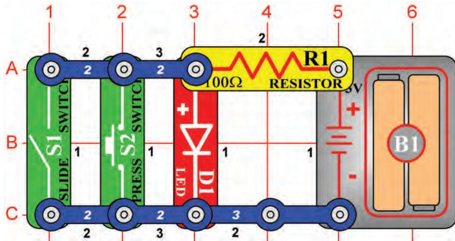
Build the circuit at left and test the combinations of the slide switch (S1) and press switch (S2). If you compare it to the OR circuit in Project #47, you can see the LED lights in the opposite combinations of that circuit. Hence, we refer to it as a NOR circuit (short for “NOT this OR that”). Like the OR and AND, it is an important building block in computers.
