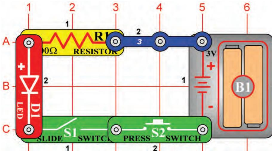
Build the circuit shown. Notice that if you turn on the slide switch (S1) AND press the press switch (S2) the LED (D1) lights up. Once again, there is no partially lit state here, the LED is either totally on or totally off. Two switches like this may be used to turn on the same light in your house, the room switch and the master switch in the electrical box. You could also have more than two switches and the circuit would function the same way.
