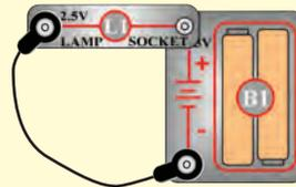
3. **Snap wires:** Use this mini-circuit to test each of the snap wires, one at a time. The lamp should light.
