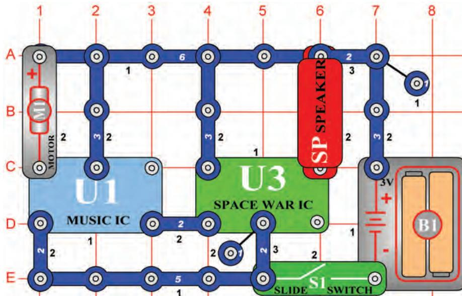
**OBJECTIVE:** To build a circuit that uses a motor to activate space war sounds.
