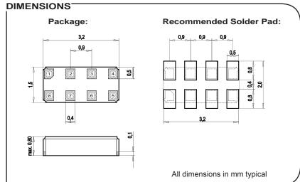
Ultra small SMT ceramic package with integrated 32.768kHz Crystal Automotive qualified, according to AEC-Q200 Rev. C I<sup>2</sup>C Interface Address: D0h Frequency-Offset Trimming Register Programmable Alarm and Interrupt Oscillator Fail Detection Watchdog Timer Programmable Clock-Output
