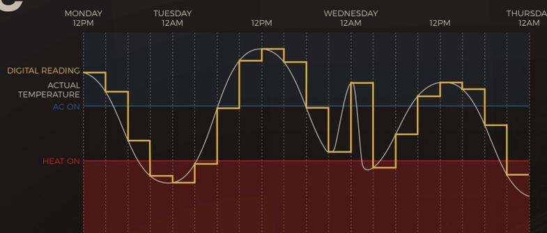
**HERE WE'VE TAKEN THE SAME TEMPERATURE DATA**, but doubled the sample rate of the digital sensor, resulting in much more accurate heating and cooling and hopefully, a more comfortable home.
