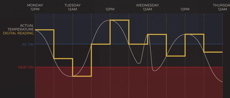
**IN THIS EXAMPLE**, the sensor is taking heat readings every six hours. We see that while the digital readings generally follow the curve of the actual temperature, it doesn't always get it quite right and sometimes misses important details, like the unexpected spike in heat on Wednesday morning.
