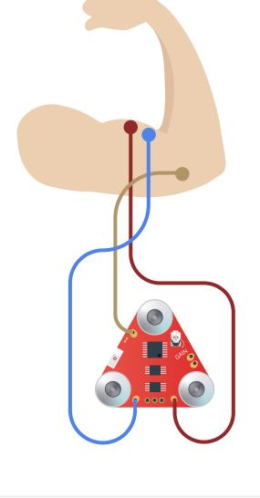
muscle body Middle Connect this pad to the cable leading to an electrode placed in the middle of the
