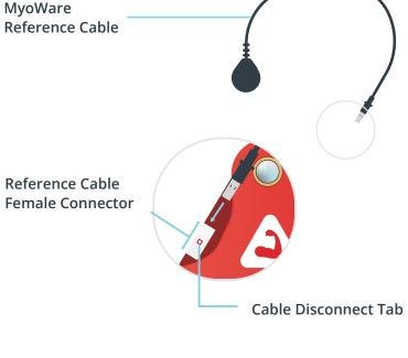
Cable into the female connector located on the left side of the sensor. Remove the cable by pressing
