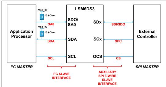
Figure 23. External controller connection in Mode 3
