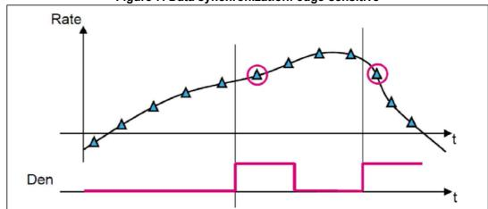
Figure 7. Data synchronization: edge-sensitive
