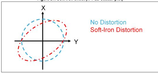
Figure 21. Soft-iron effect (X-Y 2D scatter plot)
