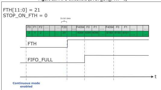
Figure 29. FIFO threshold (STOP\_ON\_FTH = 0)
