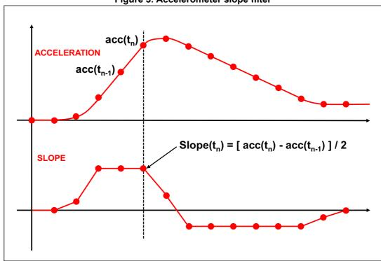
Figure 3. Accelerometer slope filter
