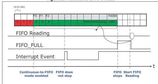
Figure 26. Continuous-to-FIFO mode
