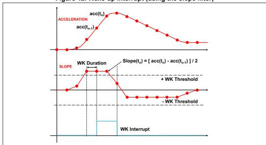
Figure 12. Wake-up interrupt (using the slope filter)
