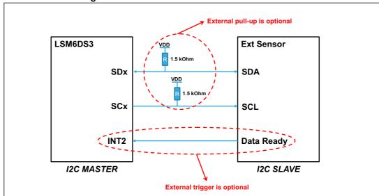
Figure 18. External sensor connections in Mode 2
