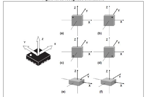
Figure 13. 6D recognized orientations
