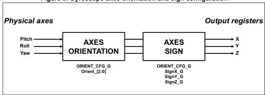
The Orient\_[2:0] bits of the ORIENT\_CFG\_G register allows driving the pitch, roll and yaw physical axes to the X, Y and Z output registers as indicated in *Table 23*.
