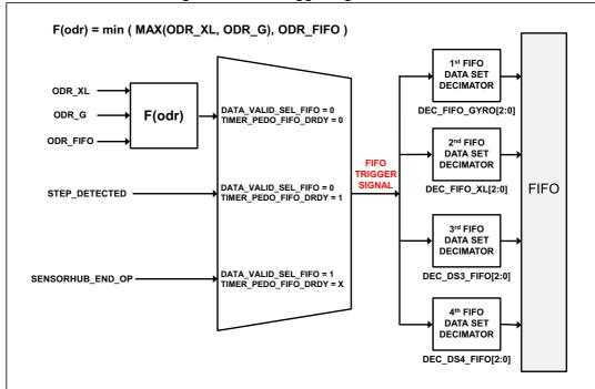
Figure 28. FIFO trigger signal selection
