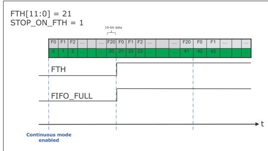
Figure 30. FIFO threshold (STOP\_ON\_FTH = 1) in Continuous mode
