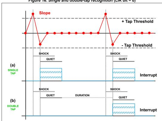
Figure 16. Single and double-tap recognition (LIR bit = 0)
