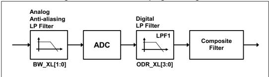
The analog signal coming from the mechanical parts is filtered by a low-pass anti-aliasing filter before being converted by the ADC. The anti-aliasing filter is enabled in High-Performance mode only.
