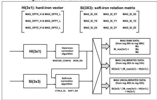
Figure 22. Hard-iron / soft-iron correction block scheme
