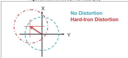
Figure 20. Hard-iron effect (X-Y 2D scatter plot)
