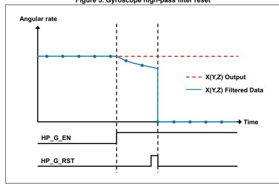
Figure 5. Gyroscope high-pass filter reset
