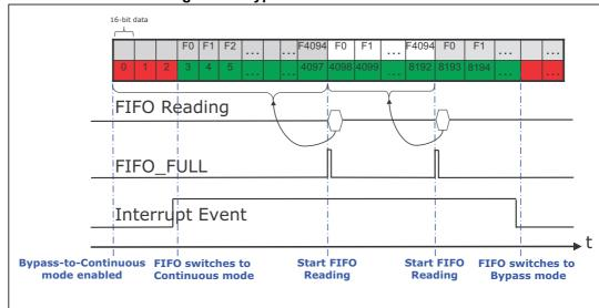
Figure 27. Bypass-to-Continuous mode
