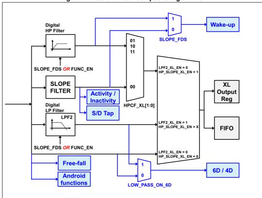
Figure 2. Accelerometer composite digital filter
