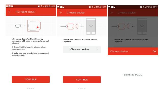
Follow the prompts and choose the Blynk board you have plugged in. You may need to reconfigure the board by holding down the "0" button for 4 second (it should blink white while you hold the button down). Once you do so it should generate a new color code.
