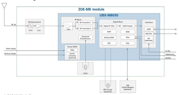
Figure 1: ZOE-M8 block diagram
