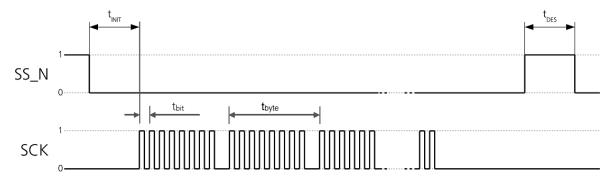
Figure 4: SPI timing diagram
