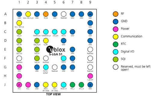
Figure 2: Pin assignment of ZOE-M8G (S-LGA51), top view
