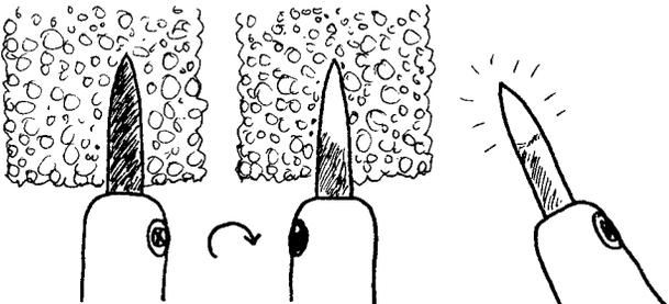
THIS SHOULD MAKE THE TIP SILVERY AND SOMEWHAT SHINY - READY TO SOLDER. REMEMBER TO CLEAN THE TIP LIKE THIS BEFORE EACH CONNECTION YOU MAKE - THE TIPS OXIDIZE QUICKLY! IF THE TIP IS NICE AND SILVERY AND SHINY, YOU CAN MAKE GOOD CONNECTIONS.
