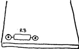
SINCE THE WORD "RESISTOR" STARTS WITH THE LETTER "R", THE PCB USUALLY MARKS PLACES WHERE RESISTORS GO WITH AN "R", FOLLOWED BY THE RESISTOR'S NUMBER, SUCH AS "R3".
