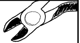
PLACE THE FLAT EDGE DOWN, PARALLEL TO THE PCB, JUST AT THE TOP OF THE LITTLE BUMP OF SOLDER. SQUEEZE THE HANDLES, AND THE CUTTING EDGES SNAP SHUT.
