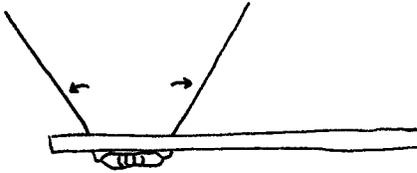
THEN YOU BEND THE LEADS OF THE RESISTOR OUTWARDS AT ABOUT 45 DEGREES SO THE PART WON'T FALL OUT WHILE WE SOLDER IT IN PLACE.
