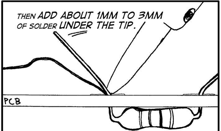
DON'T ADD IT ABOVE THE TIP, SINCE THAT MELTS THE SOLDER ONLY ONTO THE TIP, WHERE IT DOESN'T DO ANY GOOD. WE WANT THE SOLDER TO FLOW NICELY ALL AROUND BOTH THE PAD AND THE LEAD TO MAKE A GOOD CONNECTION.
