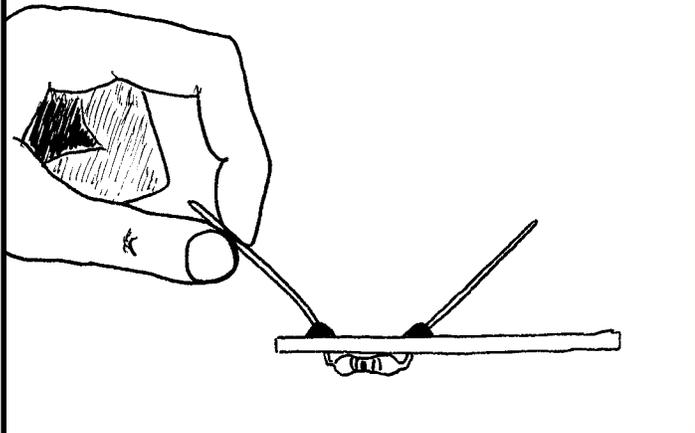
IF THE EXCESS LEAD IS TOO SHORT TO HOLD ONTO (BUT LONG ENOUGH TO POTENTIALLY SHORT OUT TO SOMETHING ON YOUR PCB), THEN POSITION THE WIRE CUTTER, HOLD YOUR FINGERS OVER THE LEAD,
