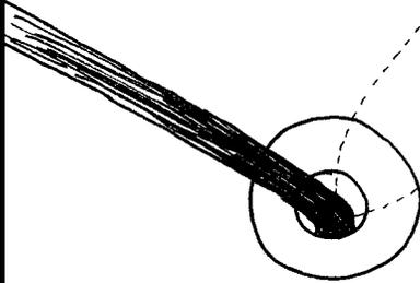
THEN ADD ABOUT 1MM TO 3MM OF SOLDER UNDER THE TIP.
