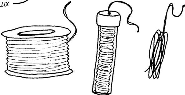
THERE ARE OTHER TYPES, FOR INSTANCE LEAD-FREE SOLDER, BUT IT HAS TOXIC CHEMICALS IN ITS CORE, AND IT IS NOT QUITE AS EASY TO USE AS SOLDER WITH LEAD. IT ALSO CORRODES SOLDERING IRON TIPS QUICKLY. IF YOU CAN ONLY GET LEAD-FREE SOLDER WHERE YOU LIVE, IT'S OK, BUT PLEASE DON'T BREATHE IN THE NASTY SMOKE.
