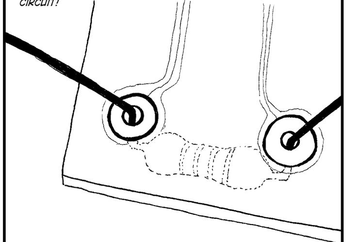
IF YOU PUT ALL OF THE LEADS FROM THE PARTS INTO THE CORRECT PADS FOR THE PARTS AND IF YOU PUT ALL OF THE PARTS IN THE CORRECT ORIENTATION AND IF YOU MAKE ALL GOOD SOLDER CONNECTIONS
