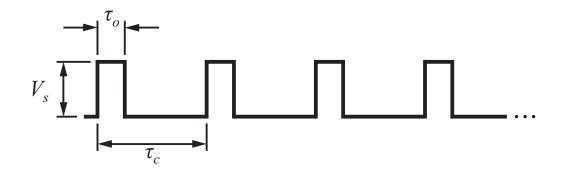
The effective voltage is  $V_{\rm eff}=V_s \frac{\tau_o}{\tau_c}$   $\frac{\tau_o}{\tau_c}$  is called the duty cycle
