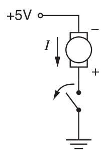
Inductive behavior of the motor causes current to continue to flow when the switch is opened suddenly.
