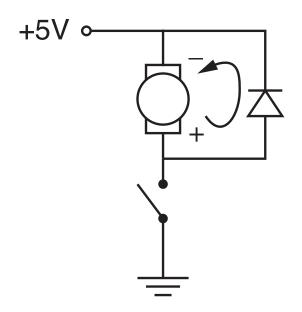
The flyback diode allows charge to dissipate without arcing across the switch, or without flowing back to ground through the +5V voltage supply.
