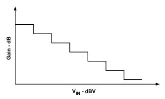
Figure 26. Input Signal Voltage vs Gain
