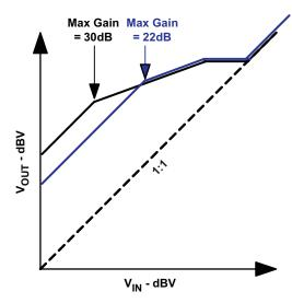
Figure 33. Output Signal vs. Input Signal State Diagram Showing Different Maximum Gains
