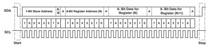
Figure 36. Typical I<sup>2</sup>C Sequence
