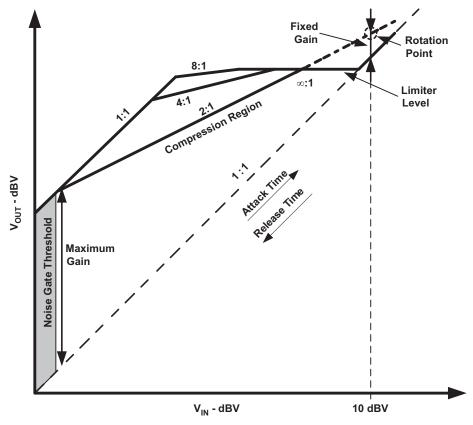
Figure 35. Output Signal vs. Input Signal State Diagram
