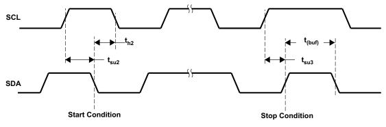
Figure 2. Start and Stop Conditions Timing
