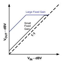
Figure 29. Output Signal vs. Input Signal State Diagram Showing Same Limiter Level Configurations with Different Fixed Gain Configurations
