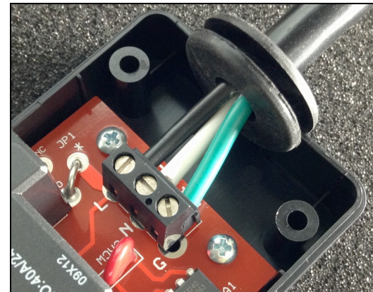
Figure 1 Line side cords attached with optional terminal block J2. Upper: European. Lower: US/Canada
