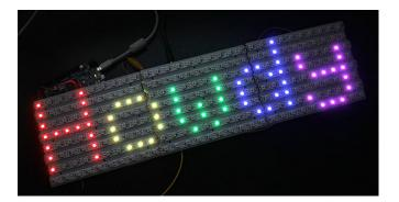
The Adafruit\_NeoMatrix library builds upon Adafruit\_NeoPixel to create two-dimensional graphic displays using NeoPixels. You can then easily draw shapes, text and animation without having to calculate every X/Y pixel position. Small NeoPixel matrices are available in the shop. Larger displays can be formed using sections of NeoPixel strip, as shown in the photo above.
