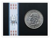
**NeoPixel Digital RGB LED Weatherproof Strip:** 30 LEDs per meter on a white backing strip.
