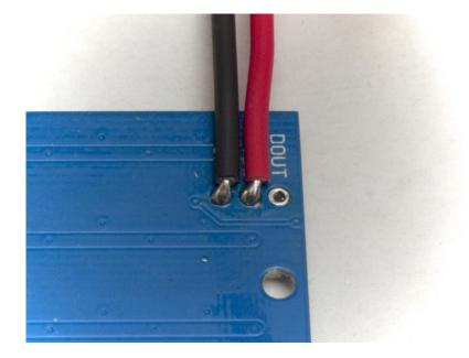
Alright! Now we can power our LEDs. Next, we need to get data from the Fadecandy Controller to the NeoMatrix. Just like power, we need two wires for data. The positive wire (DIN) carries video data, and the negative wire (GND) completes the circuit.
