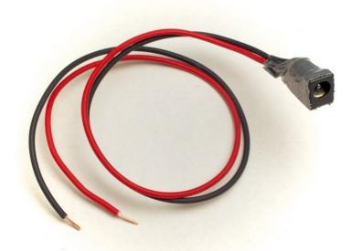
These wires will go to the VDD and GND pins on the NeoMatrix. Since we'll need a GND pin for the Fadecandy board too, it's convenient to attach these wires to the side of the NeoMatrix with DOUT instead of DIN.
