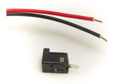
If you have multiple colors of wire, the tradition is to use black or green for ground and red or another bright color for positive. I used red and black wire. This wire should be relatively thick, since it has to carry several amps of power. I used 20 gauge stranded wire.
