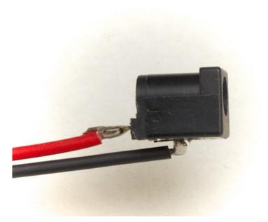
The barrel jack is almost ready to use! You'll want to insulate it, though, so you don't have to worry about metal objects bridging the two power terminals. It's especially important to watch out for short circuits when you're using such a large power supply!
