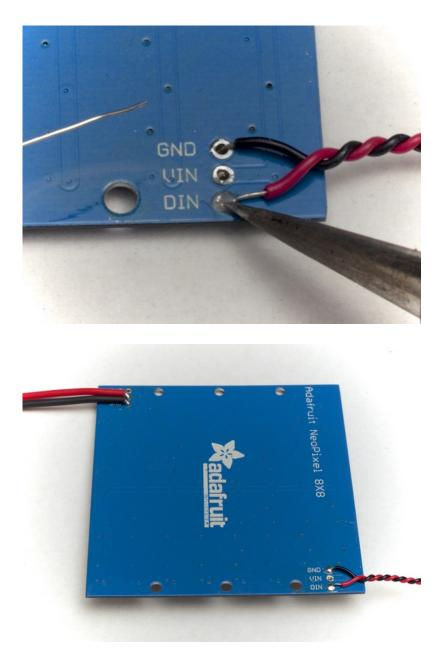
The other end of this wire pair connects to channel Zero on the Fadecandy Controller. The GND wire needs to connect to the - terminal on the Fadecandy, and the DIN wire connects to +. There are tiny + and - labels on the board, or you can remember that the pins nearest to the edge are all -.
