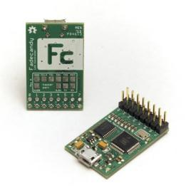
Fadecandy works with any WS2811 or WS2812 LEDs, and you can program your LEDs using many different environments. This tutorial covers one particular LED module and one particular programming environment. We'll be programming an 8x8 NeoMatrix (http://adafru.it/1487) in the Processing (http://adafru.it/cV8) language.
