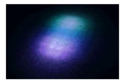
The paper acts like a rear-projection screen. In signal processing terms, it's also acting like a low-pass filter (http://adafru.it/cWb) or blur. The hard edges of each LED are filtered out, and the result looks much more like what appears on-screen.
