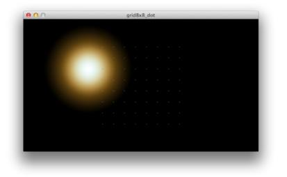
The large orange glowing dot follows your mouse. Each of the tiny single-pixel dots represents one of your 64 LEDs. With Fadecandy's Processing library, it's easy to create effects that draw to the screen and sample specific on-screen pixels for each LED.
