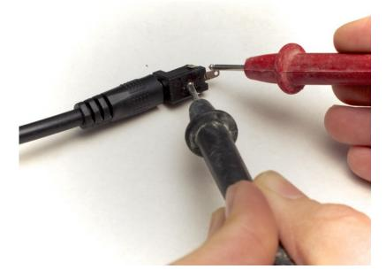
Following the polarity on the diagram above, we'll put the black probe on the pin that attaches to the outside casing of the plug, and the red probe goes on the center pin. If all is well, you should see a positive number close to 5V.
