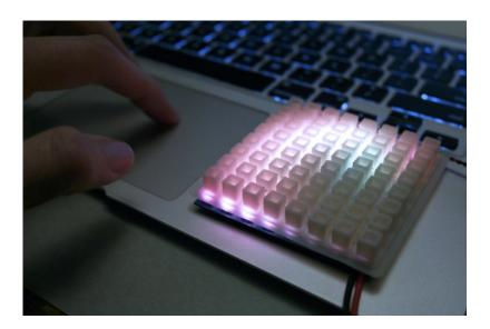
Individually addressable LEDs are everywhere. In the quest for a smaller, cheaper, smarter LED, the latest and hottest technology is the NeoPixel (http://adafru.it/cVZ), AdaFruit's term for the **WS2812**. This is an amazing little chip that integrates red, green, and blue LEDs with a controller chip into a single package.
