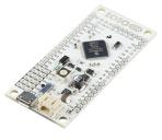
The IOIO-OTG can act as either a host or an accessory, depending on what it's connected to. Below is a brief explanation of each connection scheme and how it works:
