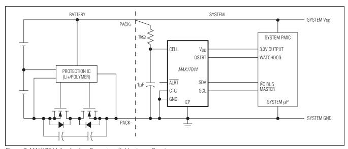
Figure 7. MAX17044 Application Example with Hardware Reset
