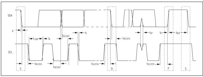
Figure 1. 2-Wire Bus Timing Diagram
