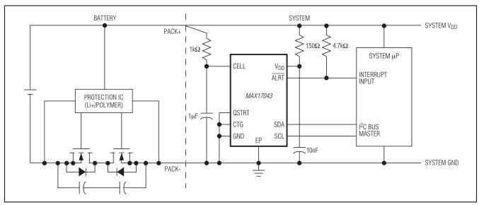
Figure 6. MAX17043 Application Example with Alert Interrupt
