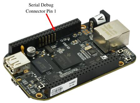
Figure 54 Serial Debug Header
