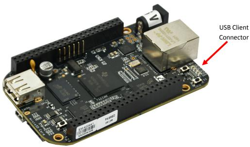
Figure 52 USB Client Connector
