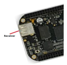
Figure 10 Connect Keyboard and Mouse Receiver to the Board
