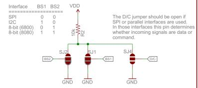
In I2C mode, D/C sets the lower bit of the 7-bit address. Short it one way or the other.
