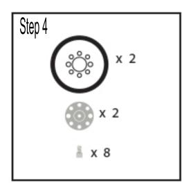
Feed four screws through each wheel and into the threaded holes of the of the set screw hub on the other side. Make sure the set screw faces away from the wheel.
