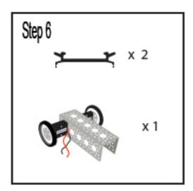
Snap the Arduino mounts onto the channel using the idicated holes. These mounts can be rearranged for different applications if desired.
