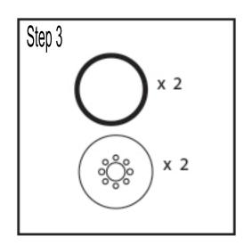
Stretch the rubber lip ring over the edge of the 2" precision disk wheels so that the wheel is evenly covered by the ring.
