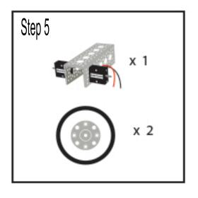
Slide the wheels onto the motor output shaft so that the set screw faces in toward the motor. Use the provided hex head driver to tighten the set screws. When tightening the set screws make sure that they sit centered on the flat portion of the motors output shaft.
