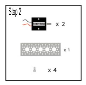
Insert 4 screws into the indicated holes from the inside of the channel. Using the provided hex head driver fasten the gearmotors to the channel with their wiring facing back toward the long side of the channel.
