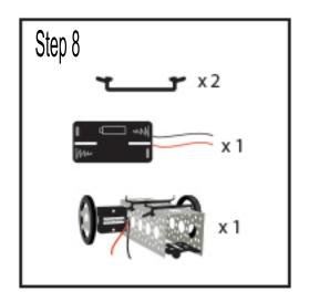
Slide the AA battery pack inside the channel. Snap the acetal battery mounts into the indicated holes to hold the battery pack in place.
