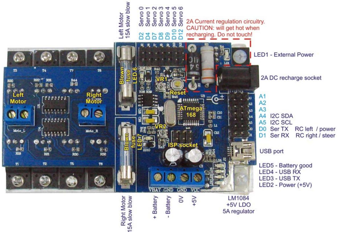
The Wild Thumper robot controller is an AVR / Arduino compatible controller that offers enthusiast the ability to get their robot up and running quickly and easily. Although relatively small in size this controller is packed with features:
