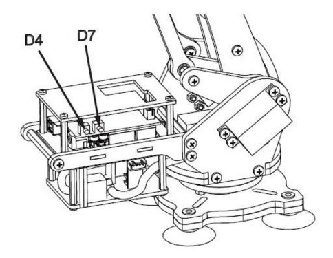
(1) Press D4 once, after one short beep you should be able to easily move the arm forward, backward, up and down. The uArm is in recording (learning) mode and the Arduino board will record the movements of the uArm.
