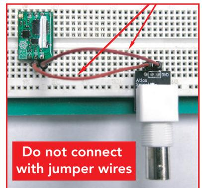
The Atlas Scientific™ EZO™ class conductivity circuit is a piece of sensitive equipment. Debugging should be done in a bread board; Not like what is show in this photo.
