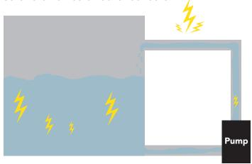
When electrical noise is interfering with the pH readings it is common to see rapidly fluctuating readings or readings that are consistently off. To verify that electrical noise is causing inaccurate readings place the pH probe in a cup of water by itself. The readings should stabilize quickly, confirming that electrical noise was the issue.
