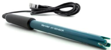
Our pH Sensor can be used for any lab or demonstration that can be done with a traditional pH meter, including: acid-base titrations, monitoring pH in an aquarium, and investigating the water quality of streams and lakes.
