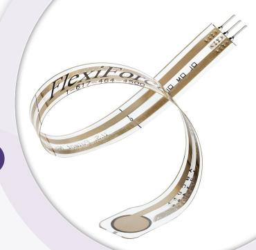
The FlexiForce A201 is our standard sensor and meets the requirements of most customers. The A201 is a thin and flexible piezoresistive force sensor that is available off-the-shelf in a variety of lengths for easy proof of concept. These ultra-thin sensors are ideal for non-intrusive force and pressure measurement in a variety of applications. This sensor is designed to use with your own electronics or multimeter.
