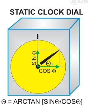
CLOCK DIAL ROTATING CLOCKWISE AT RATE  $\boldsymbol{\omega}$
