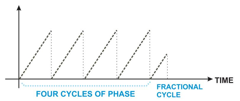
**TOTAL PHASE = 4 CYCLES + FRACTION OF CYCLE**
