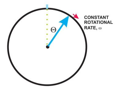
ROTARY CLOCK PHASE CAN BE EXPRESSED IN CYCLES, RADIANS, DEGREES, SECONDS, MINUTES, HOURS, 1UNIT(0 to 1), etc...
