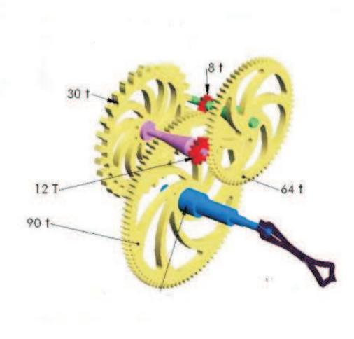
$\omega n = \omega m / GEAR RATIO$
