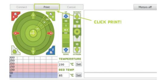
**10B** Your LulzBot TAZ will first cool down and move to the front of the bed to clean off its nozzle. After cleaning, your LulzBot TAZ will then conduct an automated bed-leveling sequence, heat up to final temperature, and start printing. This process can take up to five minutes.
