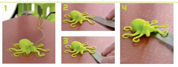
The blade is sharp, so be careful when using the blue handled knife. When in use, the knife blade should be nearly parallel with the print bed. Carefully pry away from the bed, with the sharp edge between the object and print bed.
